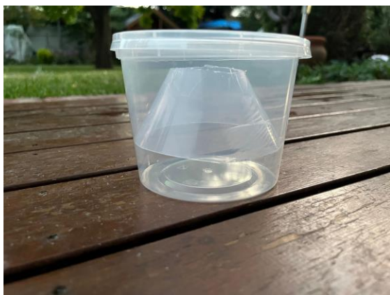
Grow larvae in an emergence container. A plastic takeaway container and cut down funnel. You can grow up mosquitoes or other insects collected in other water or soil
